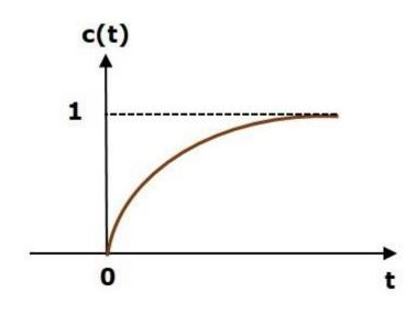
The value of the **unit step response, c(t)** is zero at t = 0 and for all negative values of t. It is gradually increasing from zero value and finally reaches to one in steady state. So, the steady state value depends on the magnitude of the input.
