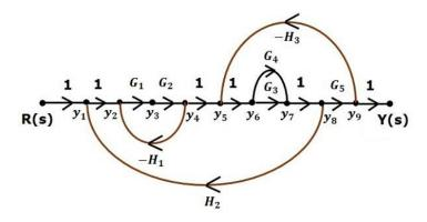
With the help of Mason's gain formula (discussed in the next chapter), you can calculate the transfer function of this signal flow graph. This is the advantage of signal flow graphs. Here, we no need to simplify (reduce) the signal flow graphs for calculating the transfer function.
