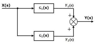
For this combination, we will get the output Y(s) as  $Y(s)=Y_1(s)+Y_2(s)$ Where,  $Y_1(s)=G_1(s)X(s)$  and  $Y_2(s)=G_2(s)X(s)$   $\Rightarrow Y(s)=G_1(s)X(s)+G_2(s)X(s)=\{G_1(s)+G_2(s)\}X(s)$ Compare this equation with the standard form of the output equation, Y(s)=G(s)X(s). Where,  $G(s)=G_1(s)+G_2(s)$ . That means we can represent the **parallel connection** of two blocks with a single
