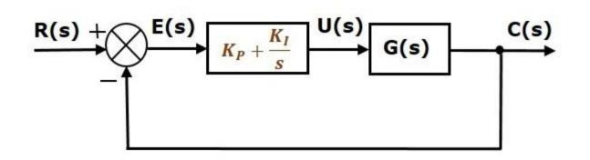
The proportional integral controller is used to decrease the steady state error without affecting the stability of the control system.
