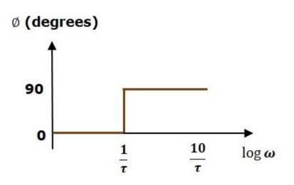
The magnitude plot is having magnitude of 0 dB upto  $\omega = 1\tau\omega = 1\tau$  rad/sec. From  $\omega = 1\tau\omega = 1\tau$  rad/sec, it is having a slope of 20 dB/dec. In this case, the phase plot is having phase angle of 0 degrees up to  $\omega = 1\tau\omega = 1\tau$  rad/sec and from here, it is having phase angle of 90<sup>0</sup>. This Bode plot is called the **asymptotic Bode plot**.
