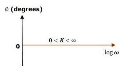
The magnitude plot is a horizontal line, which is independent of frequency. The 0 dB line itself is the magnitude plot when the value of K is one. For the positive values of K, the horizontal line will shift  $20\log K 20\log K dB$  above the 0 dB line. For the negative values of K, the horizontal line will shift  $20\log K 20\log K dB$  below the 0 dB line. The Zero degrees line itself is the phase plot for all the positive values of K.
