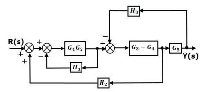
**Step 2** – Use Rule 3 for blocks  $G_1G_2$  and  $H_1$ . Use Rule 4 for shifting take-off point after the block  $G_5$ . The modified block diagram is shown in the following figure.
