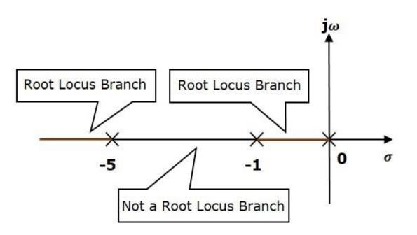
The three poles are located are shown in the above figure. The line segment between S=-1s=-1 and S=0s=0 is one branch of root locus on real axis. And the other branch of the root locus on the real axis is the line segment to the left of S=-5s=-5. **Step 2** – We will get the values of the centroid and the angle of asymptotes by using the given formulae.
