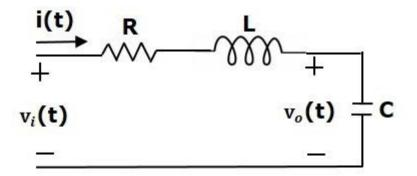
There are two storage elements (inductor and capacitor) in this circuit. So, the number of the state variables is equal to two and these state variables are the current flowing through the inductor, i(t)i(t) and the voltage across capacitor,  $v_c(t)v_c(t)$ .
