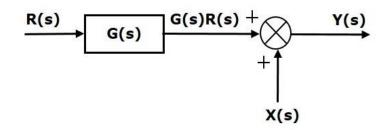
Output of the block G(s) is G(s)R(s). The output of the summing point is
