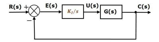
The integral controller is used to decrease the steady state error.
