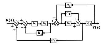
**Step 1** – Use Rule 1 for blocks  $G_1$  and  $G_2$ . Use Rule 2 for blocks  $G_3$  and  $G_4$ . The modified block diagram is shown in the following figure.
