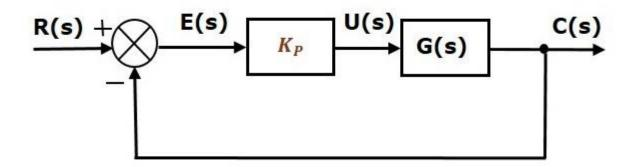
The proportional controller is used to change the transient response as per the requirement.
