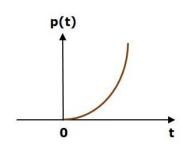
So, the unit parabolic signal exists for all the positive values of 't' including zero. And its value increases non-linearly with respect to 't' during this interval. The value of the unit parabolic signal is zero for all the negative values of 't'.
