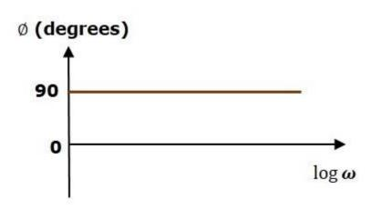
The magnitude plot is a line, which is having a slope of 20 dB/dec. This line started at  $\omega = 0.1 \omega = 0.1 \text{ rad/sec}$  having a magnitude of -20 dB and it continues on the same slope. It is touching 0 dB line at  $\omega = 1 \omega = 1 \text{ rad/sec}$ . In this case, the phase plot is 90° line.
