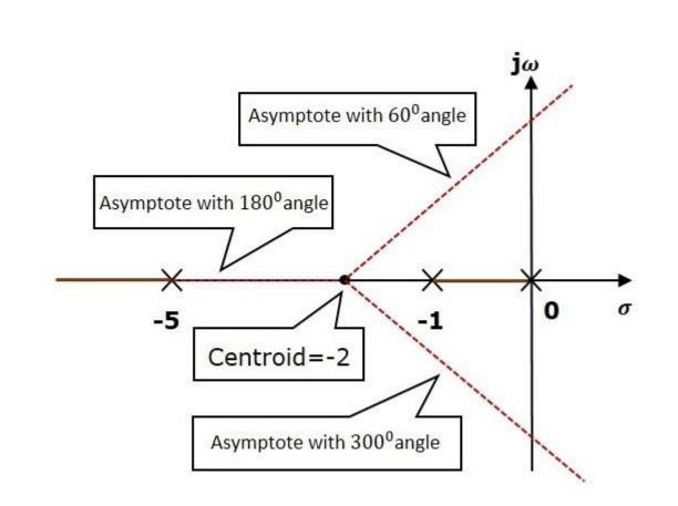
Step 3 – Since two asymptotes have the angles of 600600 and 30003000, two root locus branches intersect the imaginary axis. By using the Routh array method and special case(ii), the root locus branches intersects the imaginary axis at  $j5 - \sqrt{j5}$  and  $-j5 - \sqrt{-j5}$ .
