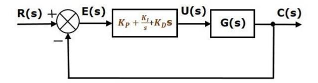
The proportional integral derivative controller is used to improve the stability of the control system and to decrease steady state error.
