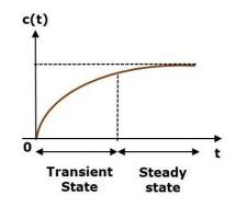
Here, both the transient and the steady states are indicated in the figure. The responses corresponding to these states are known as transient and steady state responses.
