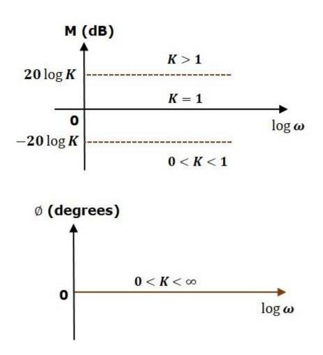
The magnitude plot is a horizontal line, which is independent of frequency. The 0 dB line itself is the magnitude plot when the value of K is one. For the positive values of K, the horizontal line will shift 20logK20log K dB above the 0 dB line. For the negative values of K, the horizontal line will shift 20logK20log K dB below the 0 dB line. The Zero degrees line itself is the phase plot for all the positive values of K.
