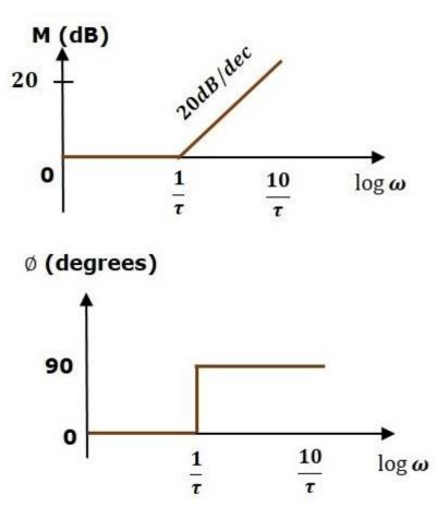
The magnitude plot is having magnitude of 0 dB upto  $\omega =_{1\tau\omega} =_{1\tau} \text{ rad/sec}$ . From  $\omega =_{1\tau\omega} =_{1\tau} \text{ rad/sec}$ , it is having a slope of 20 dB/dec. In this case, the phase plot is having phase angle of 0 degrees up to  $\omega =_{1\tau\omega} =_{1\tau} \text{ rad/sec}$  and from here, it is having phase angle of 90°. This Bode plot is called the **asymptotic Bode plot**.
