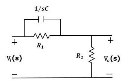
Here, the capacitor is parallel to the resistor  $R_1R_1$  and the output is measured across resistor  $R_2$ . The transfer function of this lead compensator is -
