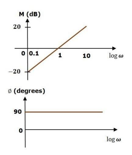
The magnitude plot is a line, which is having a slope of 20 dB/dec. This line started at  $\omega=0.1 \omega=0.1 \text{ rad/sec}$  having a magnitude of -20 dB and it continues on the same slope. It is touching 0 dB line at  $\omega=1\omega=1 \text{ rad/sec}$ . In this case, the phase plot is 90<sup>0</sup> line.
