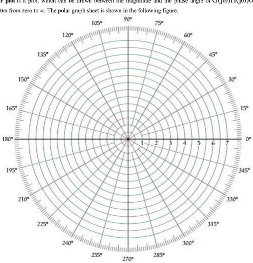
This graph sheet consists of concentric circles and radial lines. The concentric circles and the radial lines represent the magnitudes and phase angles respectively. These angles are represented by positive values in anti-clock wise direction. Similarly, we can represent angles with negative values in clockwise direction. For example, the angle  $270^{\circ}$  in anti-clock wise direction is equal to the angle  $-90^{\circ}$  in clockwise direction.
