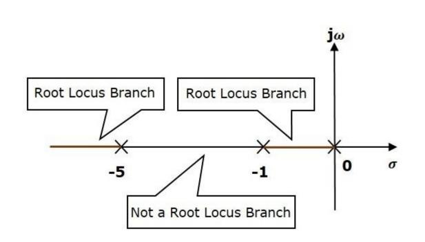
The three poles are located are shown in the above figure. The line segment between s=-1s=-1 and s=0s=0 is one branch of root locus on real axis. And the other branch of the root locus on the real axis is the line segment to the left of s=-5s=-5.
