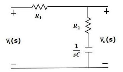
Here, the capacitor is in series with the resistor  $R_2R_2$  and the output is measured across this combination. The transfer function of this lag compensator is -
