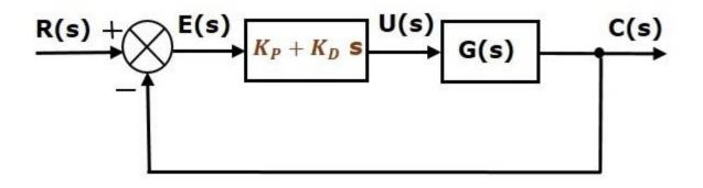
The proportional derivative controller is used to improve the stability of control system without affecting the steady state error.
