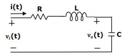
There are two storage elements (inductor and capacitor) in this circuit. So, the number of the state variables is equal to two and these state variables are the current flowing through the inductor, i(t)i(t) and the voltage across capacitor, vc(t)vc(t). From the circuit, the output voltage, v0(t)v0(t) is equal to the voltage across capacitor, vc(t)vc(t). v0(t)=vc(t)v0(t)=vc(t)
