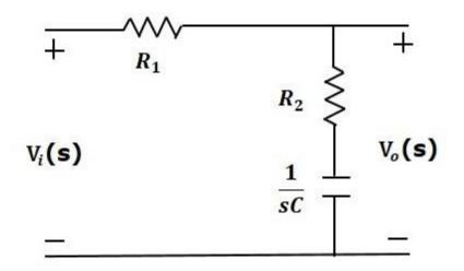
Here, the capacitor is in series with the resistor R<sub>2</sub>R<sub>2</sub> and the output is measured across this combination.
