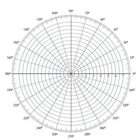
This graph sheet consists of concentric circles and radial lines. The **concentric circles** and the **radial lines** represent the magnitudes and phase angles respectively. These angles are represented by positive values in anti-clock wise direction. Similarly, we can represent angles with negative values in clockwise direction. For example, the angle  $270^{\circ}$  in anti-clock wise direction is equal to the angle  $-90^{\circ}$  in clockwise direction.
