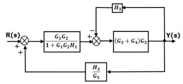
Step 4 – Use Rule 3 for blocks  $(G_3+G_4)G_5$  and  $H_3$ . The modified block diagram is shown in the following figure.
