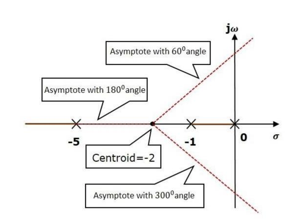
**Step 3** – Since two asymptotes have the angles of 600600 and 30003000, two root locus branches intersect the imaginary axis. By using the Routh array method and special caseiiii, the root locus branches intersects the imaginary axis at  $j5-\sqrt{j5}$  and  $-j5-\sqrt{-j5}$ .
