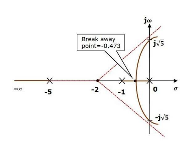
In this way, you can draw the root locus diagram of any control system and observe the movement of poles of the closed loop transfer function.
