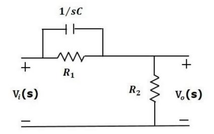
Here, the capacitor is parallel to the resistor  $R_1R_1$  and the output is measured across resistor  $R_2$ .
